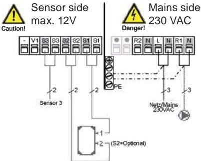
**Caution!** When S2 is installed = S1 is switch on sensor and S2 switch off sensor.
