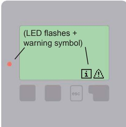
If the controller detects a malfunction, the red light flashes and the warning symbol also appears in the display. If the error is no longer present, the warning symbol changes to an info symbol and the red light no longer flashes. To obtain more detailed information on the error, press the key under the warning or info symbol.
