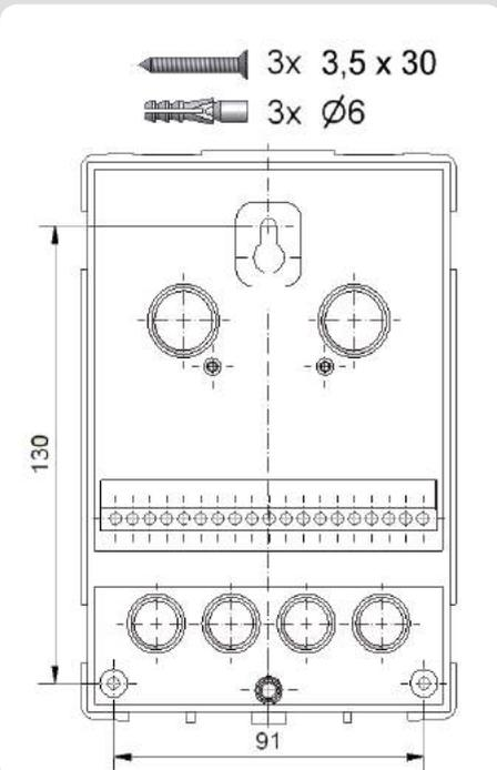
5. Using a drill and size 6 bit, drill 3 holes at the points marked on the wall and push in the plugs.
