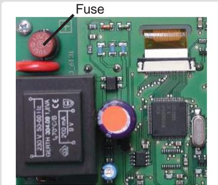
If the mains voltage is switched on and the controller still does not function or display anything, then the internal device fuse may be defective. In that case, open the device as described under C, remove the old fuse and check it.
